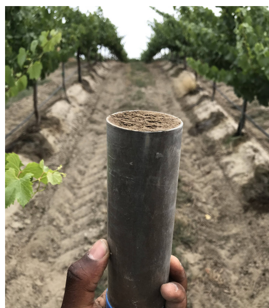
Figure 28. Soil scientists sampling soil bulk density in vineyards to quantify soil health. (Photo: Sarpong)
