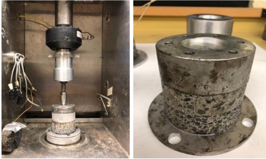
Figure 3.10. Tensile strength test of shotcrete-concrete interface bond
