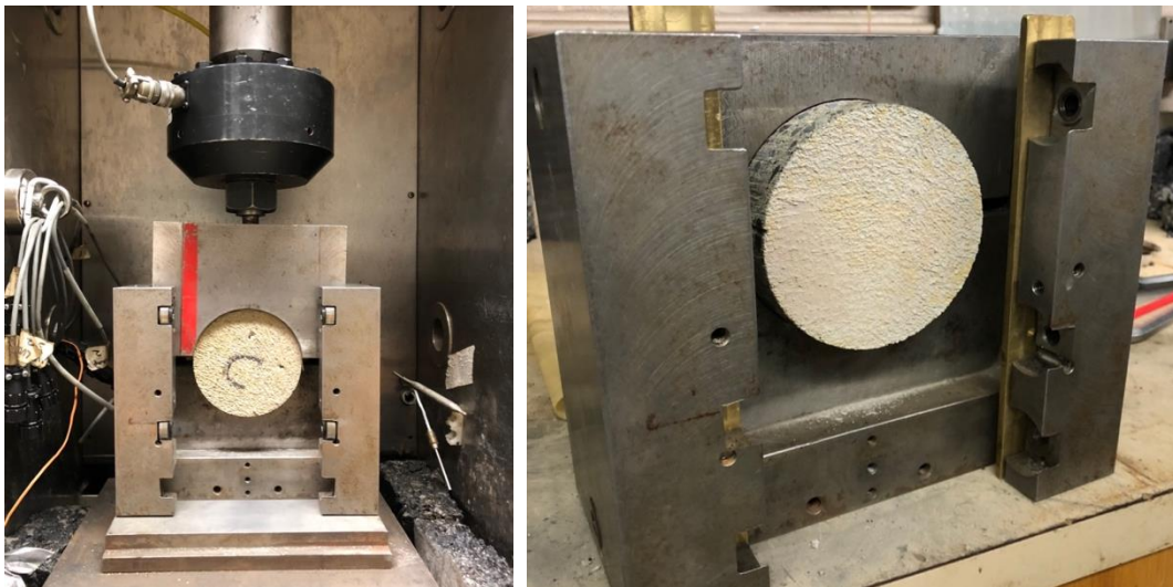
Figure 3.12 Shear strength test of shotcrete-concrete interface bond
