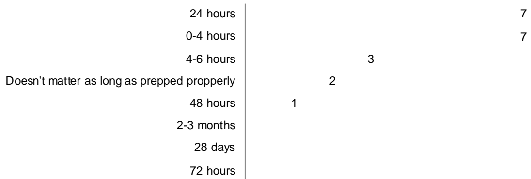
Figure 2.15 Common delay between shotcrete layers in multilayer shotcreting
