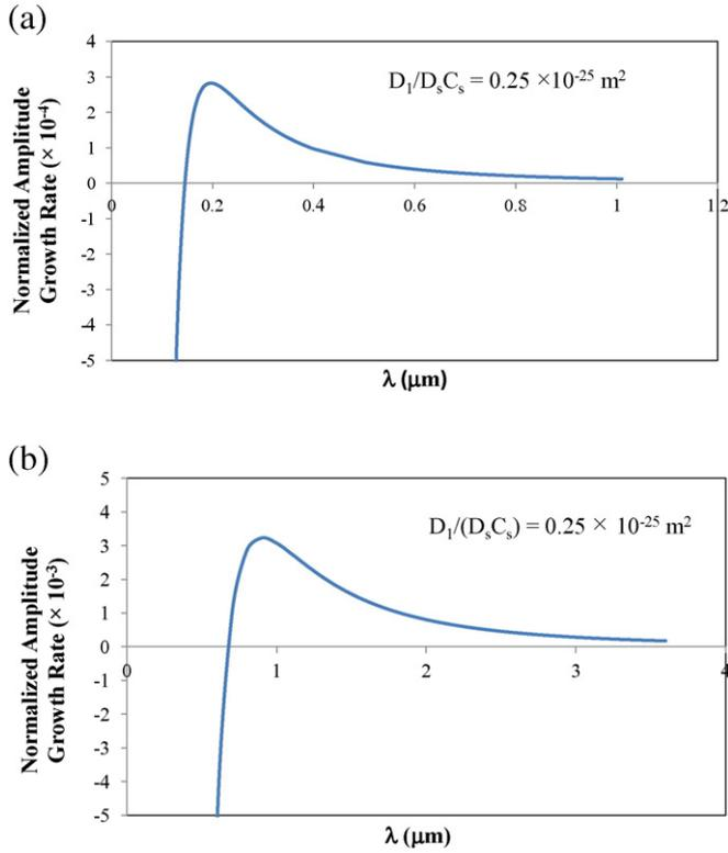
Fig. 2. Rate of growth for different surface perturbation wavelengths. (a) for 2 GPa stress and (b) for 1 GPa stress.
