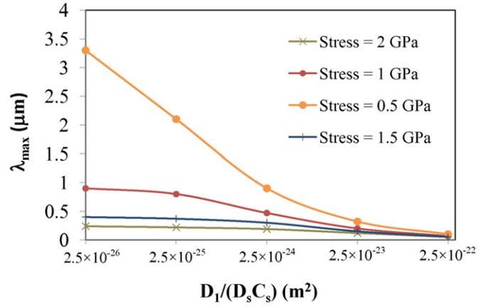
Fig. 3. The  $\lambda_{\text{max}}$  for different volume to surface diffusivity ratios at different stress levels.
