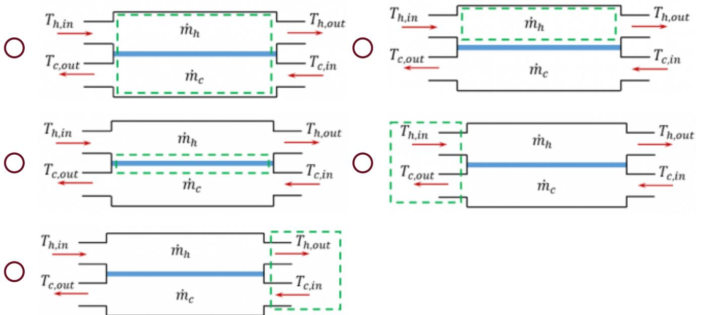
What area would you use for  $A_i$  in  $\dot{Q} = U_i A_i \Delta T_{LM}$  in a shell and tube heat exchanger?
