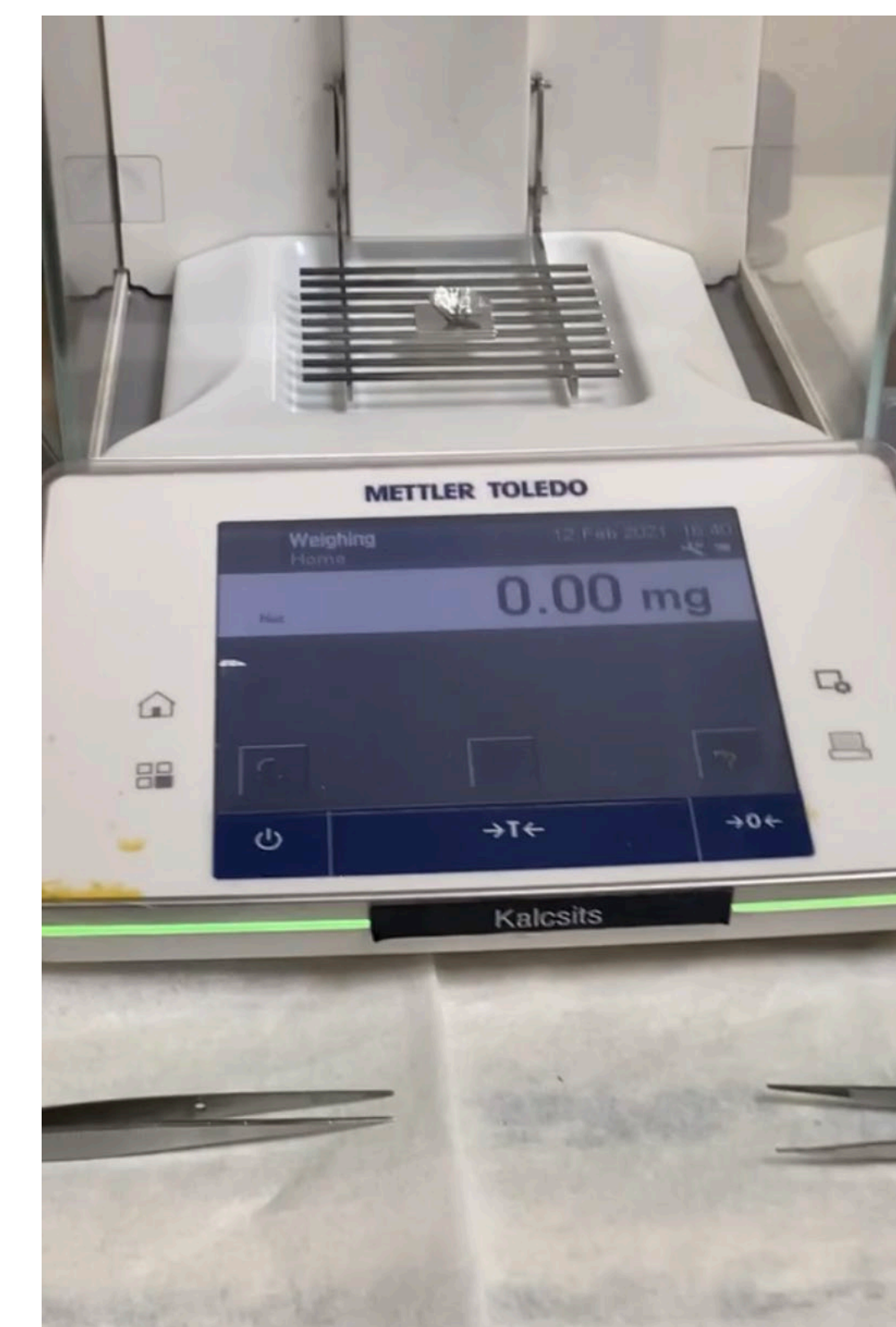
Figure 1.3 This is a photo of the scale that measures the isotope samples. Each sample must be measured in between 2.9-3.1mg. The total number of samples exceeded 600.
