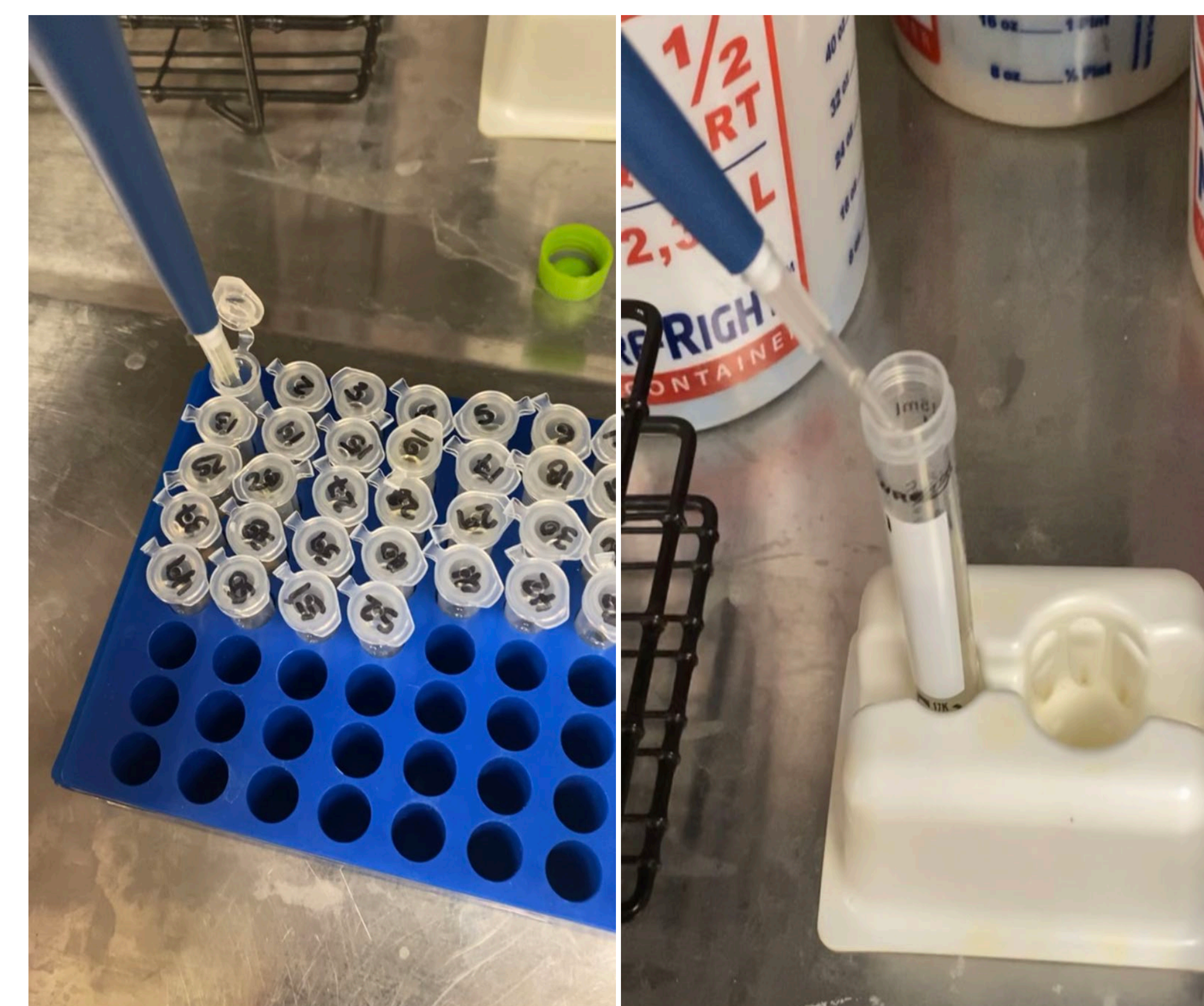
Figure 1.4 This photo is part of the procedure of preparing samples for the MP-AES. The photo left is a pipette measuring 200 microliters from a sample. The photo right is the transfer of 200 microliters into 800 microliters of deionized water. Because the sample was diluted into nitric acid, all work was under a fume hood. Protective wear such as nitrile gloves, lab coat, and eye wear was worn.
