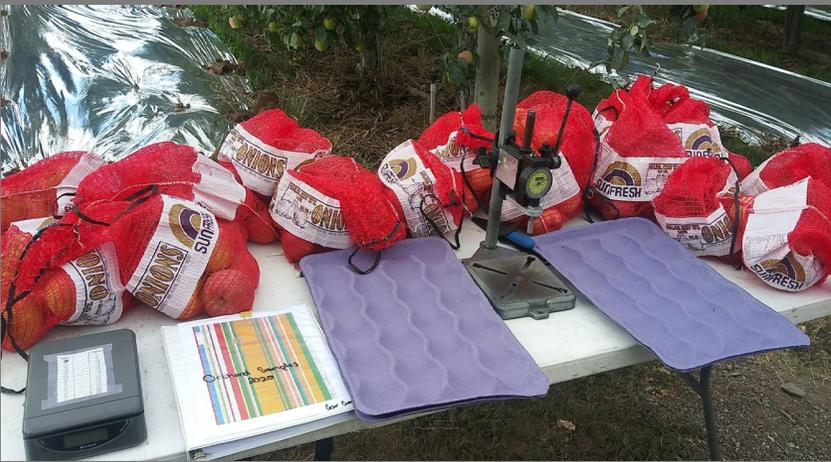
In the picture there is red bags containing apple samples that I took from different orchards as well as a scale to measure the weight of the fruit and determine the size. There is also a penetrometer which tells you the pressure of the apple once pressed.
