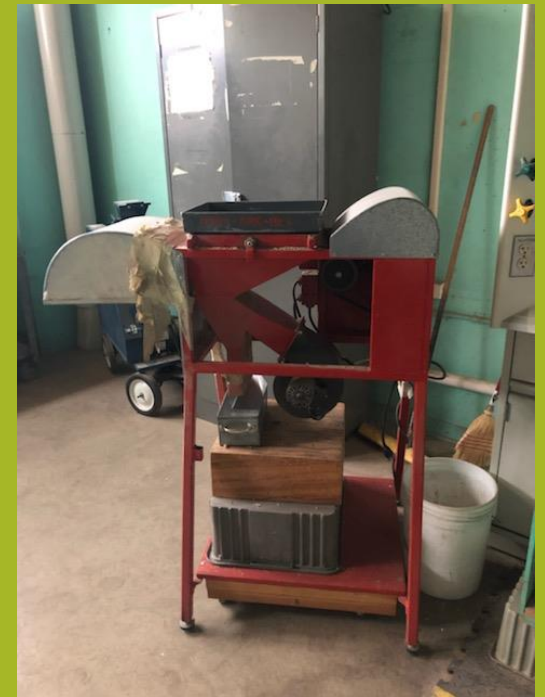
This was the seed cleaner used to clear chaff and other excess plant material from the seed.
