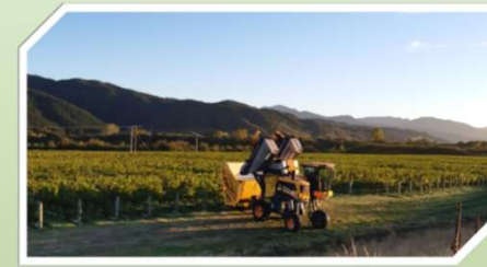
Harvester tipping harvested grapes into gondola pulled by tractor during harvest
