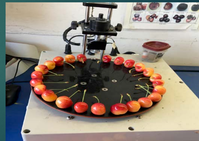
Firmtech measures size and firmness of cherries
