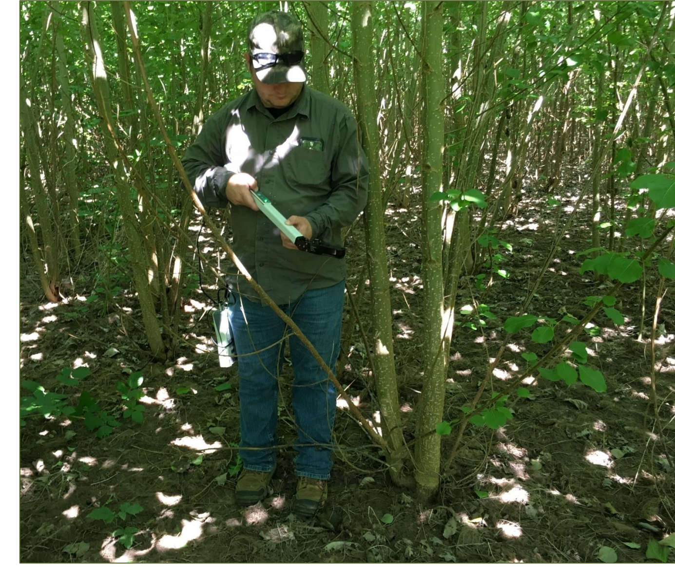
Fig. 5. Jason Mack (A) and Luke Murphy (B) taking readings below canopy using the LAI 2200C Canopy analyzer in at Jefferson
