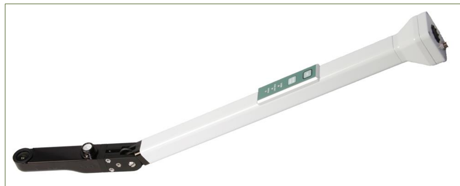
Figure 2. LAI-2250 Optical Sensor (wand) is the data collection component of the LAI-2200C. The optical sensor contains high precision optical components, including lenses, optical filters, and light sensors 1 .
