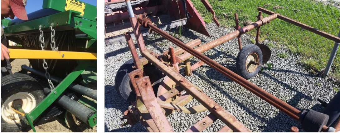
Figure 2. Feeding the mulch through the roller bar in new mulch layer (left); old mulch layer showing the rod that holds the mulch (right).
