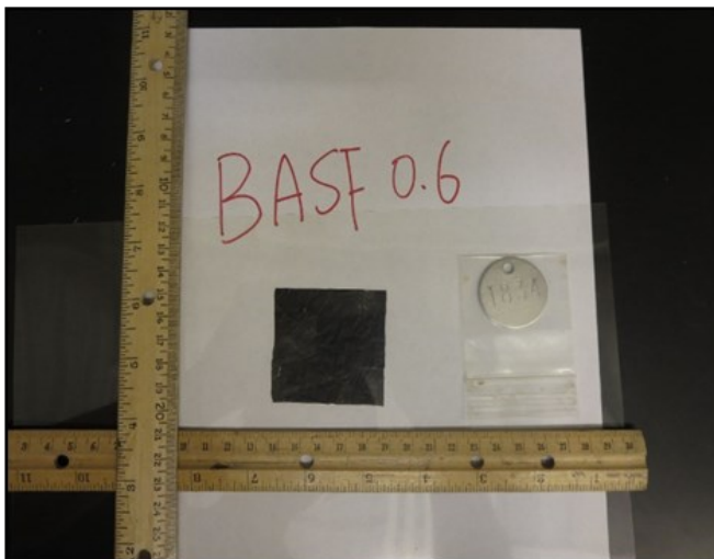
Figure 10. Mulch sample next to 2 rulers and an aluminum tag ready to be photographed.
