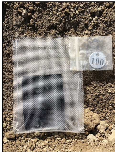
Figure 1. Mesh bag containing soil-biodegradable plastic mulch (BDM) sample can be used to estimate in-soil degradation.
