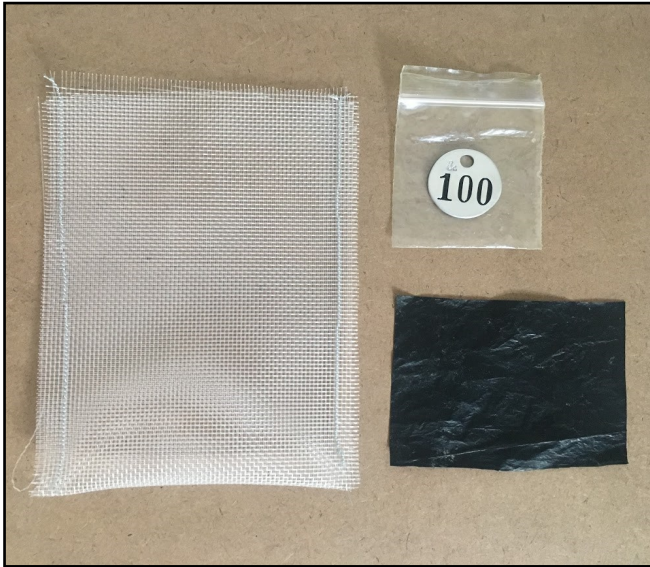
Figure 9. Mesh bag with mulch sample and aluminum tag.
