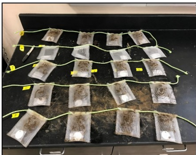
Figure 11. Mesh bags aligned with rope and stapled with stainless-steel staples.
