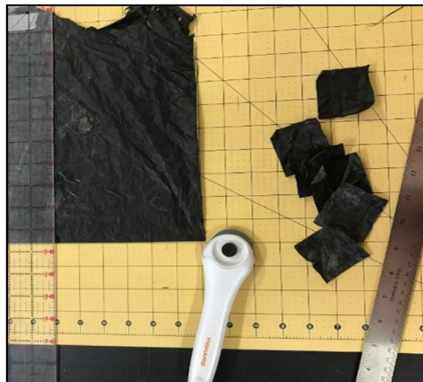
Figure 7. Mulch samples cut to 8 x 6 cm using a rotary mat and cutter.
