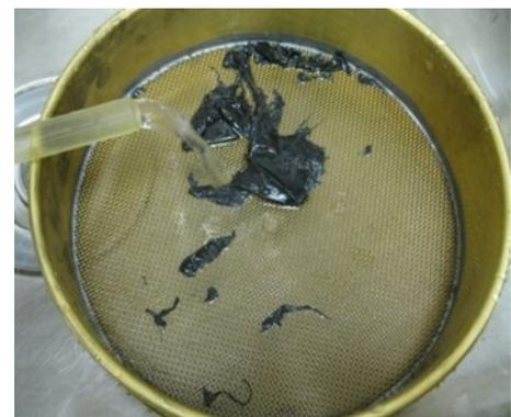
**Figure 5.** Pieces of plastic mulch on a sieve.
