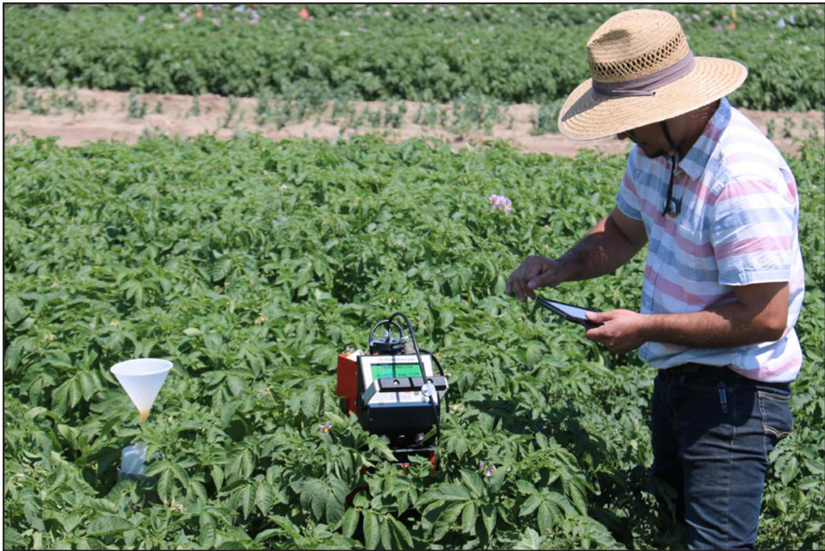
Graduate Student Francisco "Paco" Gonzalez takes a reading from his Neutron Probe in a trial measuring water use of new and existing cultivars.
