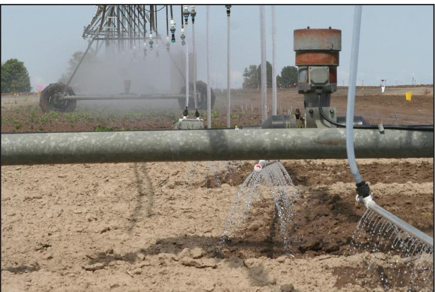
SmartDrop® booms were used to deliver different amounts of water in an irrigation study at the Othello Research Station.
