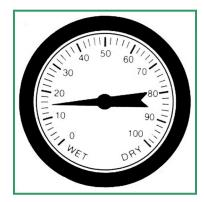
Figure 2 Tensiometer Gauge
