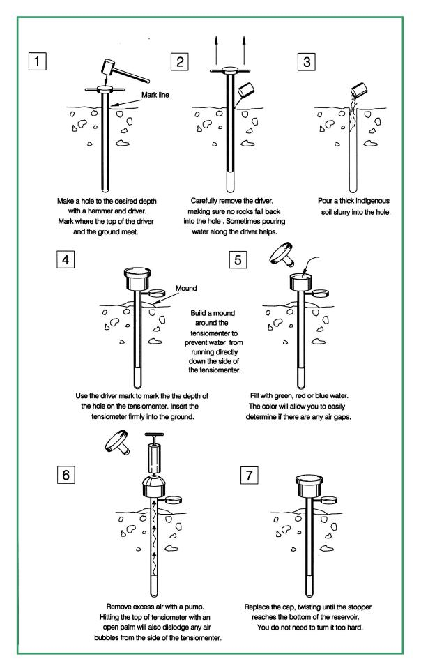
Figure 4 Tensiometer Installation Procedures
