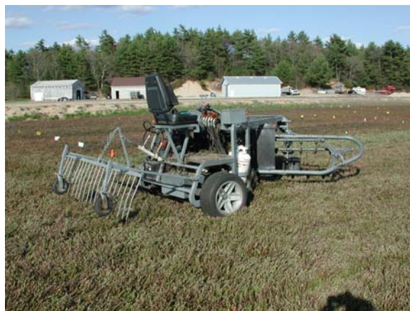
Grower-manufactured pruner with knives attached to a rotating head in front combined with a hydraulic rake attachment in the rear.
