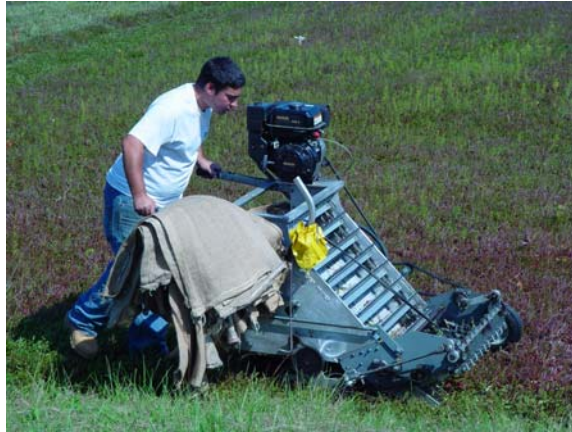
Dry harvesting with a Furford picking machine that prunes vines as well as picks fruit. Photo courtesy CCCGA.
