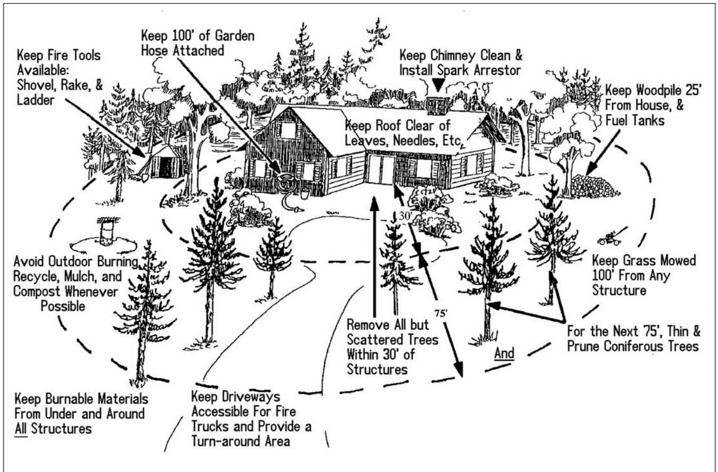
Figure 3. Structural and vegetative protection from wildfire damage
