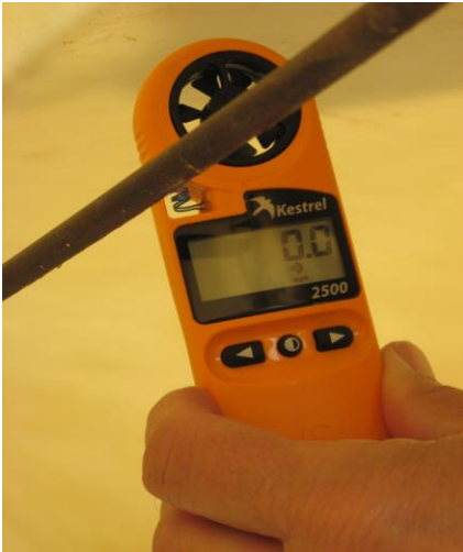
Measuring hutch airflow using an anemometer. Wind speed is zero without hutch elevation.
