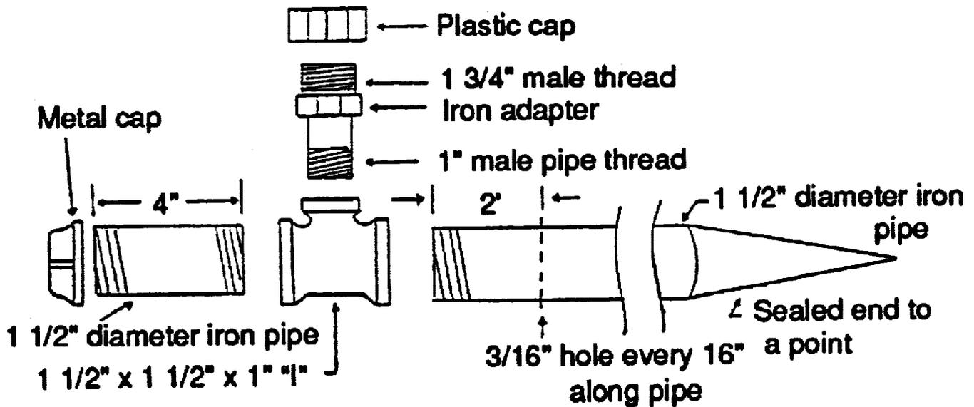
Fig. 1. Details of ammoniated pipe about 22 feet long.
