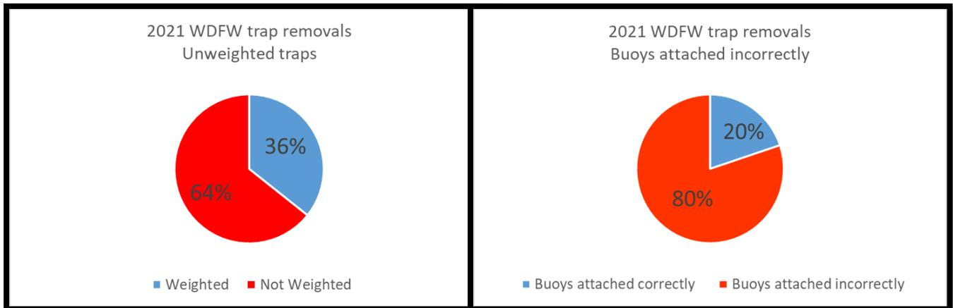
**Figure 3:** Dropping crab pots without weights and attaching buoys incorrectly contributes to derelict gear.
