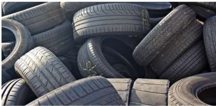
Figure 1: Tires lose about 20% of their weight during their lifetime of wear on the road. The lost material becomes chemical-laced microplastics released into the environment.
