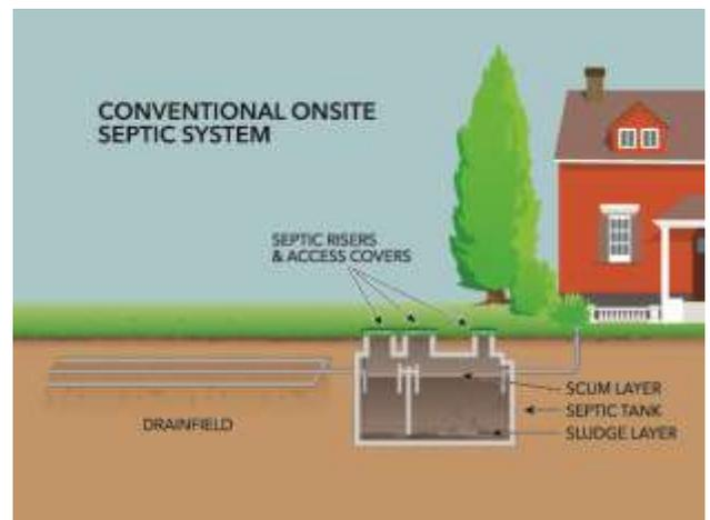
*Figure 3: Septic treatment systems also have the potential to introduce microfibers into the natural environment. While some might be captured in the tank, others could escape into the drainfield (leachfield) pipes, where they could clog soil pores or be carried into ground or surface waters. Image Credit: Shore Stewards [Guide for Shoreline Living](#).*
