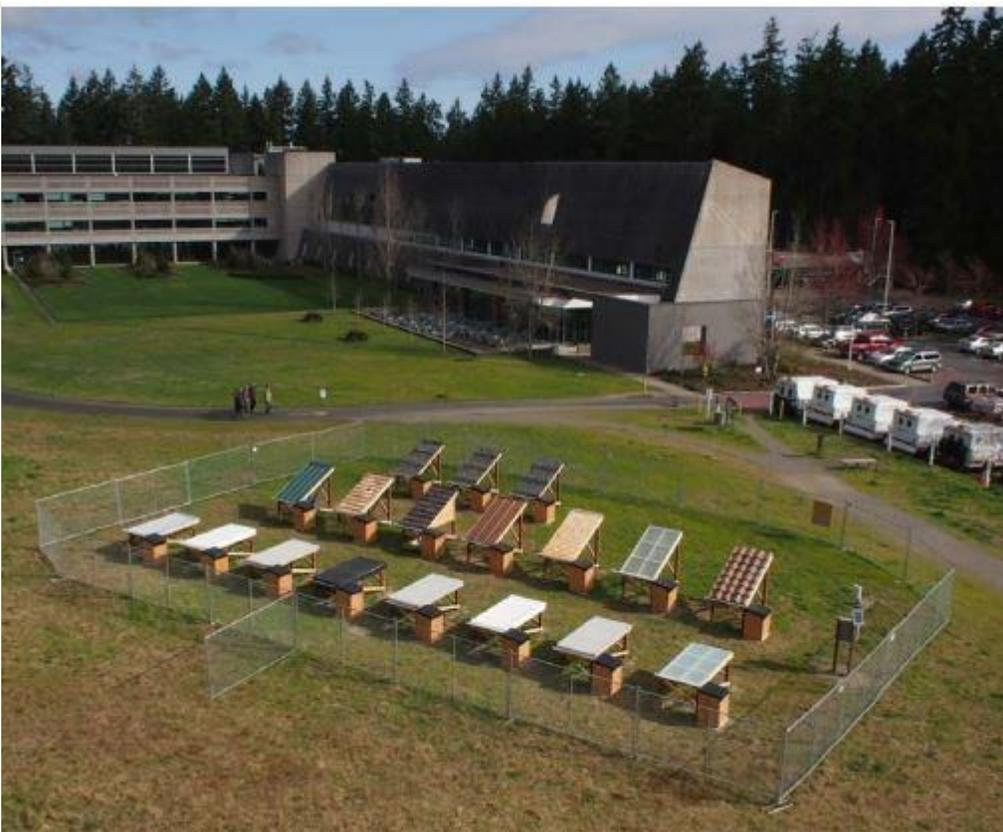
Photo of the roof runoff experiment at the Washington Department state of Ecology. [Photo of the roof runoff experiment at the Washington Department state of Ecology.](#)
