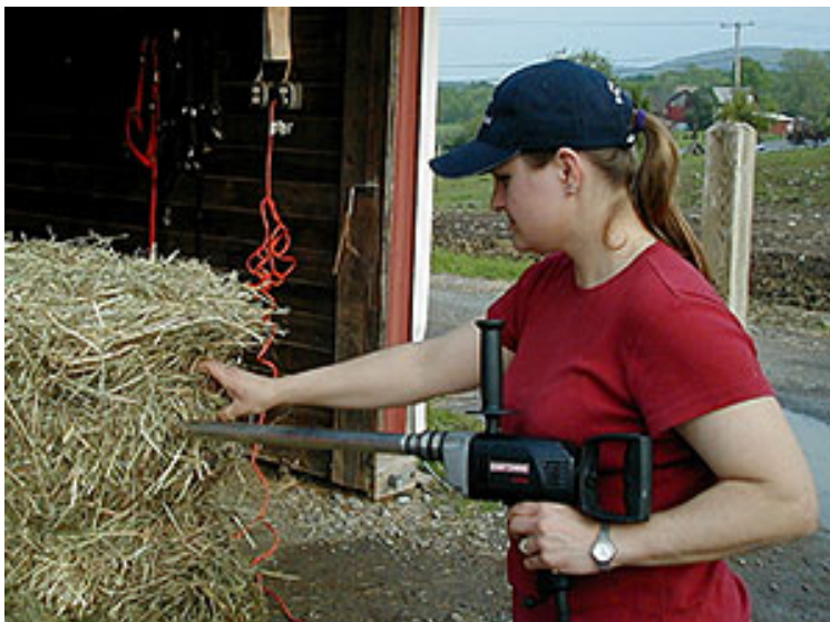
Figure 2. Drill slowly through the bale to avoid heating up the bale, thus changing the composition and moisture level. Picture from Equi-Analytical Laboratories.
