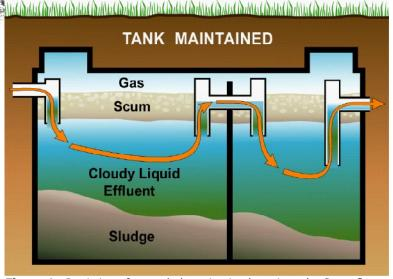
**Figure 1.** Depiction of a regularly maintained septic tank. Scum floats to the top, while sludge settles to the bottom, leaving the liquid to flow into the drainfield and be absorbed into the soil.
