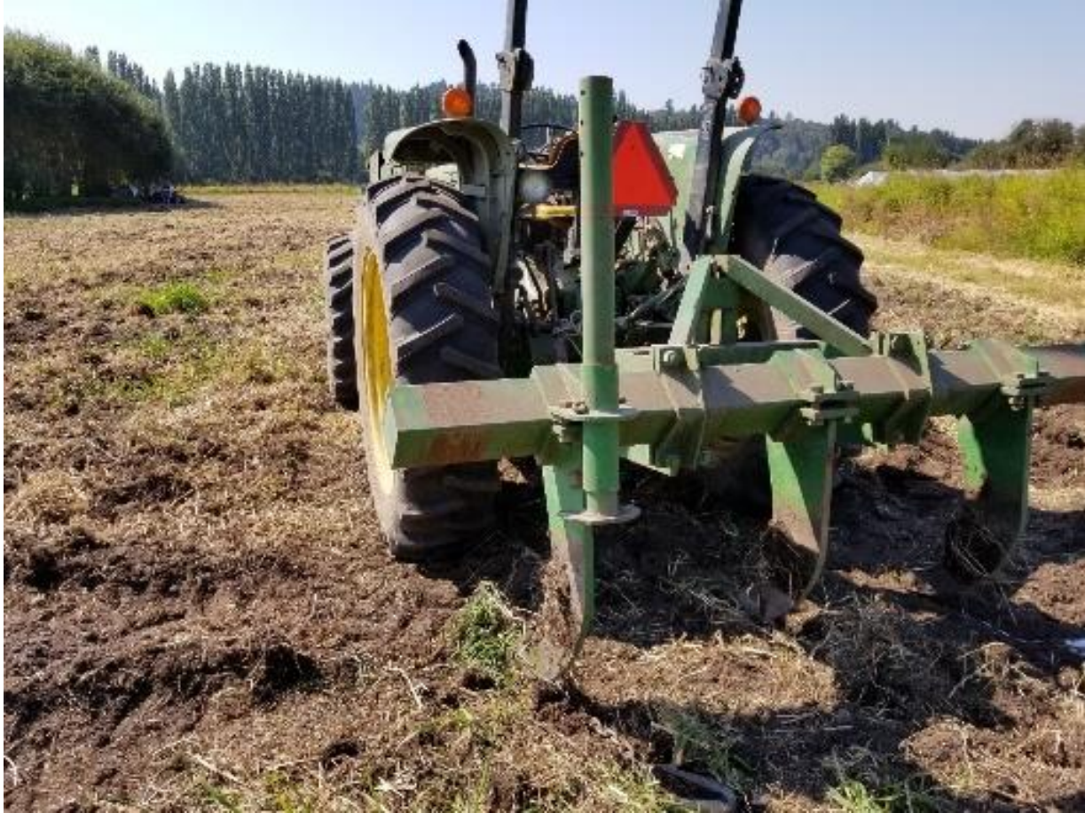
The ripper tool can reach down to three feet, but it takes a heavy-duty tractor to pull it and the process uses a lot of fuel. Photo courtesy of Viva Farms.
