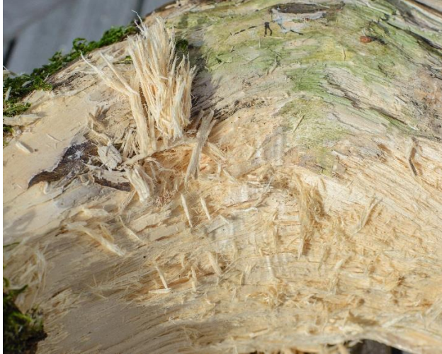
LEFT: White rot makes the wood soft, spongy and whiter than normal. Photo by Nancy Crowell.
