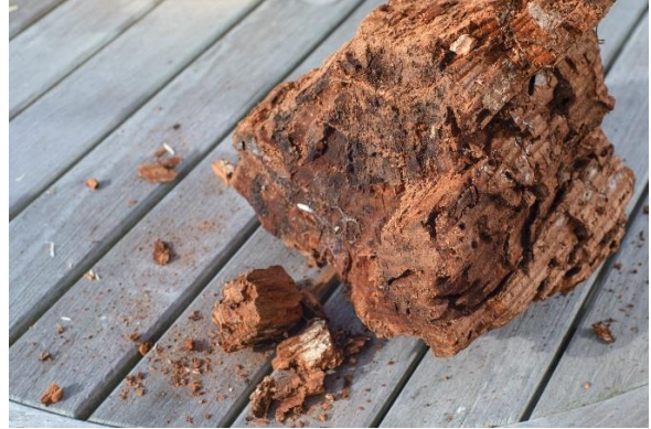
RIGHT: Brown rot creates columns or pockets of decayed wood that is dark brown, dry and fragile. Brown rot tends to crumble readily or break up into cubes of varying size. Photo by Nancy Crowell / WSU Skagit County Extension Master Gardeners.
