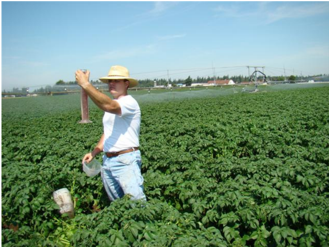
Ag. and Natural Resources Extension Agent, Don McMoran measuring the volume in a catch can with a boom irrigation system in the background.
