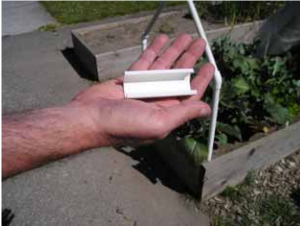
Plastic clips like this one secure row cover fabric to a framework made of PVC pipe. The clips come in two sizes to fit either 1/2-inch or 3/4-inch pipe, and are available at some gardening centers, nurseries and mail-order suppliers. Photo by Cathy Carmody.
