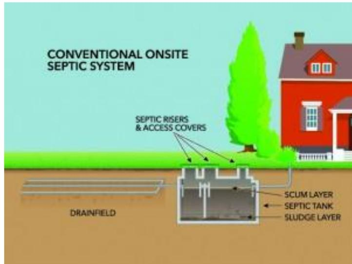
The “good” bacteria in the septic system do not completely decompose the sludge or scum layers, so the layers continue to grow, slowly filling up the tank over time. These layers will eventually need to be pumped out by a professional septic pumper. No special additives are necessary or recommended.
