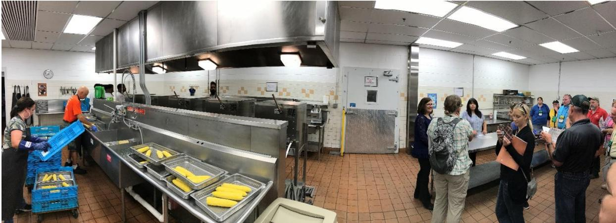
Fig. The Harry and Jeanette Weinberg Produce Preservation Center. The far side of the island houses the steam blanchers. Product is cooled in the ice bath to the left, and two ice machines are out of the frame to the left against a wall. Stainless tables to the right are used to bag and label product.
