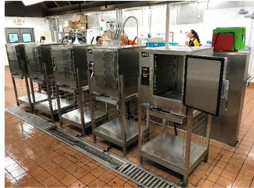
Fig. Five Accutemp Evolution Steamers with 6 hotel pan capacity. Blanch time varies from three to seven minutes. These steam units are not as fast, but eliminate the need for a much more expensive belt blancher.
