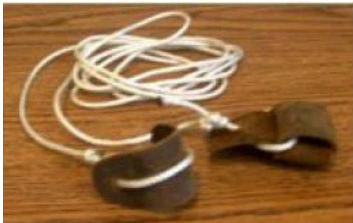
Figure 3: A completed bow stringer
