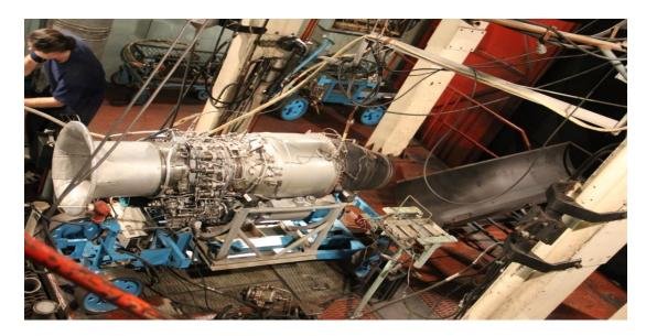
Main technical characteristics were tested: relative rotor speed n, %, engine inlet temperature  $t_{e.in.}$ , °C, barometric pressure,  $B_{atm}$ , mm Hg thrust, R, N pressure in fuel manifold,  $P_{f.m.}$ , MPa, jet pipe temperature,  $t_{j.p.}$ , °C, fuel flow, G, l/hour, acceleration response time, s.
