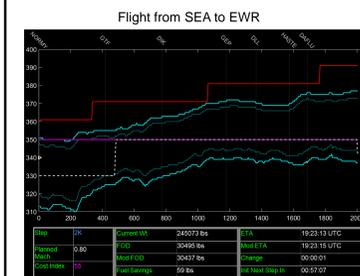
The optimal altitude is not always the max reachable altitude. In most cases, the optimal is actually below.
