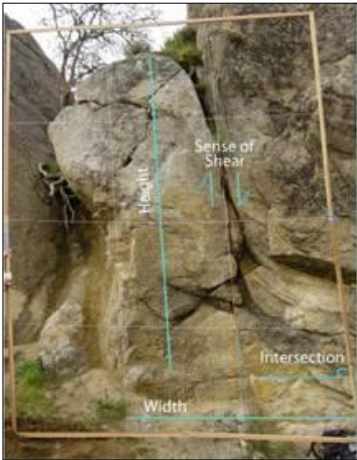
Figure 4. Vertical shear zone face showing sense of shear, height and width measurements, and the mafic layer intersection angle
