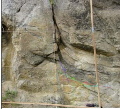
Figure 8. Vertical shear zone face with tangent lines drawn to the lower boundary of the mafic rich layer.
