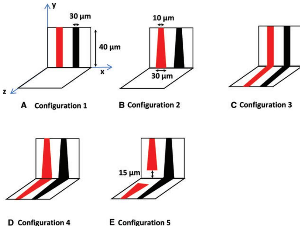
**Figure 2.** Configuration of electrodes considered for the design of the proposed separation microdevice. (A) Configuration 1: rectangular, (B) Configuration 2: trapezoidal, (C) Configuration 3: multiplane rectangular, (D) Configuration 4: multiplane trapezoidal, (E) Configuration 5: hybrid trapezoidal. Here red and black colors of the electrodes are used to differentiate the polarity of electrodes.
