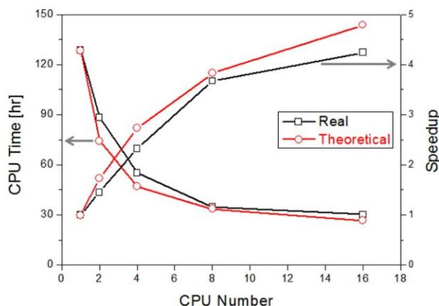
**Figure 5.** Computational time required to reach 1 s simulation time using different number of CPUs. The second vertical axis shows the speedup of the proposed algorithm. The numerical (real) speedup closely follows the theoretical speedup indicating an efficient algorithm.
