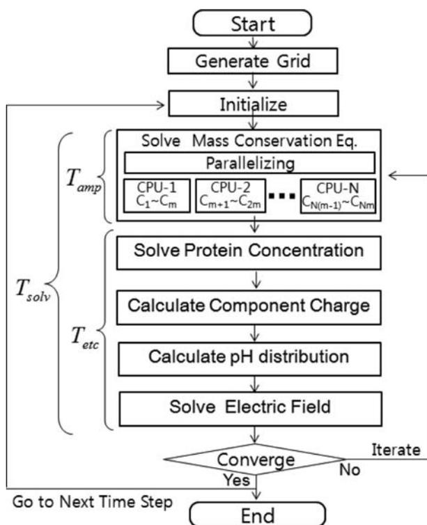
**Figure 1.** A parallel numerical algorithm for simulation of IEF using the segregated method. Only the solver for the ampholyte mass conservation equations is parallelized in this segregated scheme.
