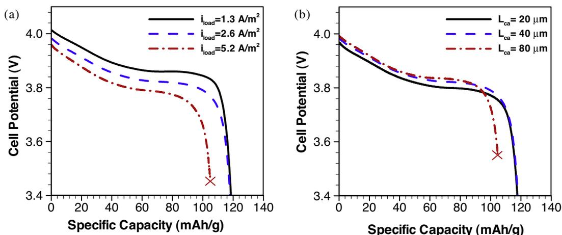
Fig. 7. Dependence of electric performance on (a) applied current density and (b) cathode thickness. All other simulation conditions are the same as in Fig. 3.
