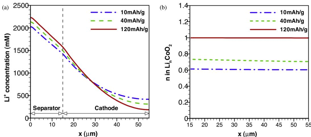
**Fig. 4.** (a) Lithium ion concentration distribution in the separator and cathode regions. (b) Changes in the cathode utilization with specific capacity. All other simulation conditions are same as in Fig. 3.
