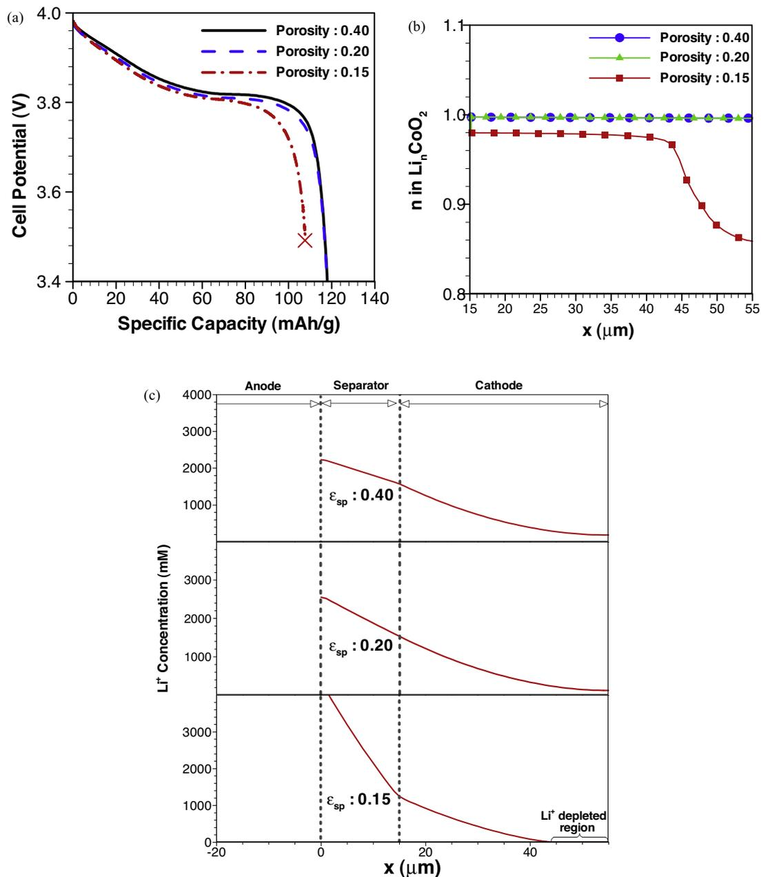
**Fig. 6.** Effect of separator porosity on the (a) electric performance of a lithium-ion battery, (b) cathode material utilization ( $n$ ) at the fully discharged state, and (c) lithium ion concentration distribution at the fully discharged state. All other simulation conditions are same as in Fig. 3.
