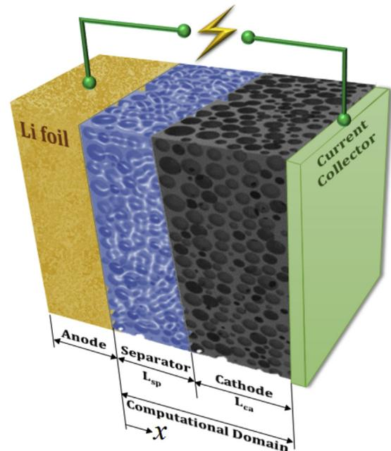
Fig. 2. Schematic of a lithium-ion battery. The computational domain ranges from the interface of anode and separator ( $x=0$ ) to the end of the cathode ( $x=L_{sp}+L_{ca}$ ).
