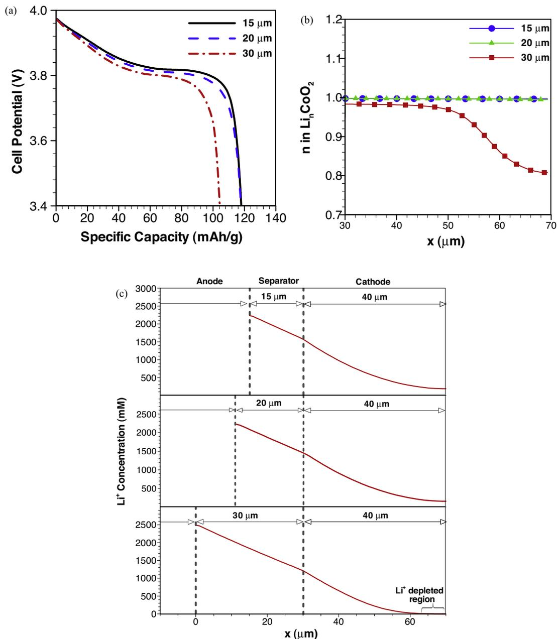
**Fig. 5.** Effect of separator thickness on the (a) electric performance of battery, (b) cathode material utilization ( $n$ ) at the fully discharged state, and (c) lithium ion concentration distribution at the fully discharged state. Here all geometric and design parameters are identical for all cases, except the separator thickness. All other simulation conditions are the same as in Fig. 3.
