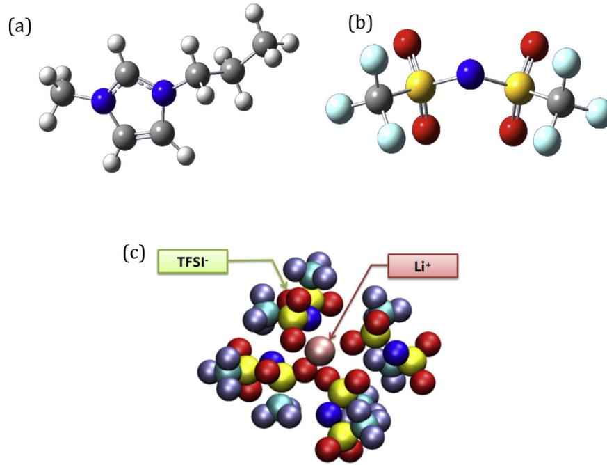
**Fig. 1.** Molecular structures of (a) mppy<sup>+</sup> (*N*-methyl-*N*-propyl pyrrolidinium) and (b) TFSI<sup>-</sup> (bis trifluoromethanesulfonyl imide). (c) Formation of cluster due to coordination of Li<sup>+</sup> with TFSI<sup>-</sup> anions in an isotropic and homogeneous liquid.
