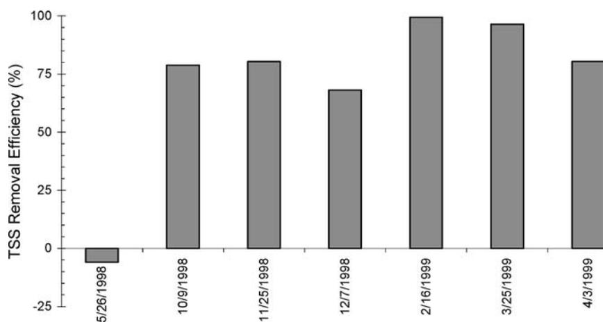
Figure 4. TSS removal efficiency for different storm events.
