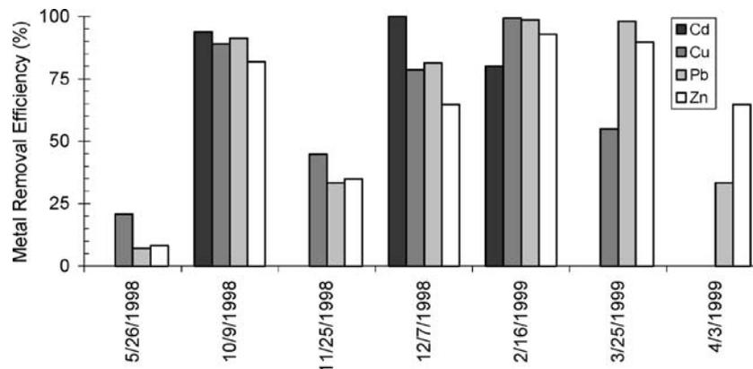
Figure 5. Metal removal efficiency for different storm events.
