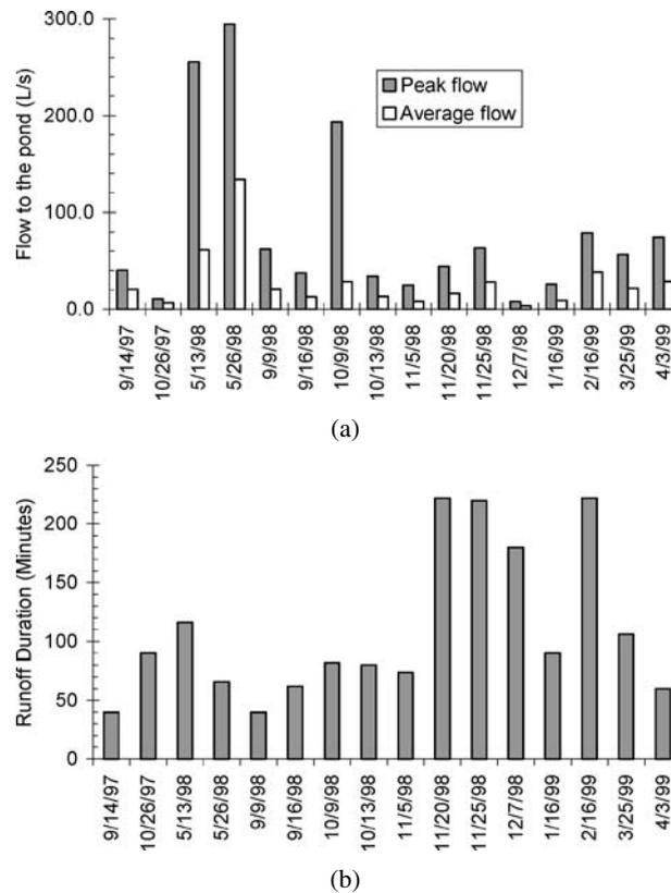
Figure 2. (a) Peak and average flow to the detention pond. (b) Duration of flow to the pond.
