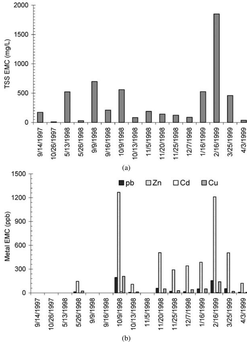
Figure 3. (a) TSS concentrations as a function of time. (b) Metal concentrations as a function of time.
