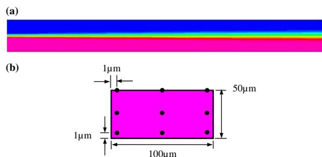
**Fig. 4** **a** The fully developed concentration field is used as the initial condition for the subsequent numerical studies; **b** initial positions of particles in the computational domain. The magnetic force is parallel to the gravity force direction
