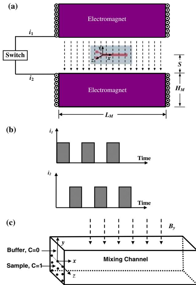
**Fig. 1** Schematic diagram of **a** magnetic micromixer; **b** time-dependent current applied to the electromagnets; **c** mixing microchannel
