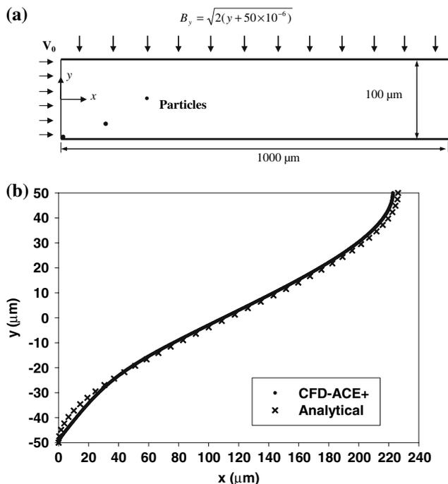
**Fig. 6** Numerical model validation: **a** schematic diagram of the 2D microchannel. The particle is initially located at the left bottom corner of the microchannel; **b** comparison of particle trajectories obtained by numerical simulation and analytical solution. Particle trajectory is recorded at every 0.2 s
