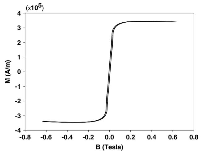
**Fig. 2** Hysteresis loop for the paramagnetic particles (Spherotech CM-10-10). Redrawn based on the original B-H hysteresis loop provided by Spherotech, Inc
