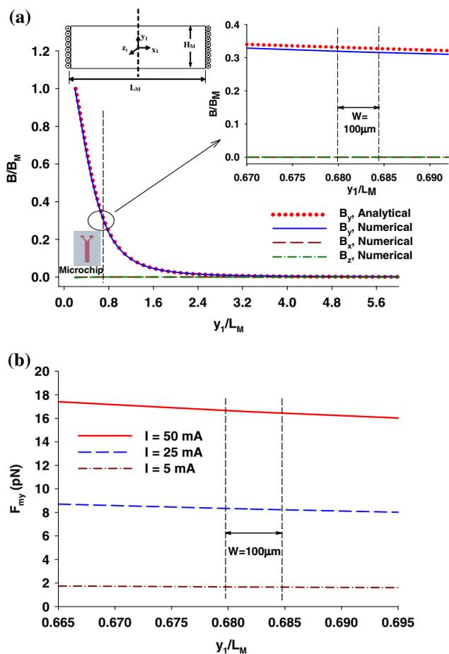
**Fig. 3** **a** Magnetic flux density generated by the electromagnet along the centerline that connects the two magnetic poles ( $z = 0$ ). The analytical solution is based on a rectangular electromagnet ( $2 \text{ cm} \times 2 \text{ cm} \times 0.8 \text{ cm}$ ). The baseline  $B_M$  is 2.27 Tesla and 2.4 Tesla for numerical and analytical solutions, respectively. Here,  $x_1 = x, y_1 = y - S - H_M/2, z_1 = z$ . **b** Magnetic actuation force exerted on the particles along the channel length
