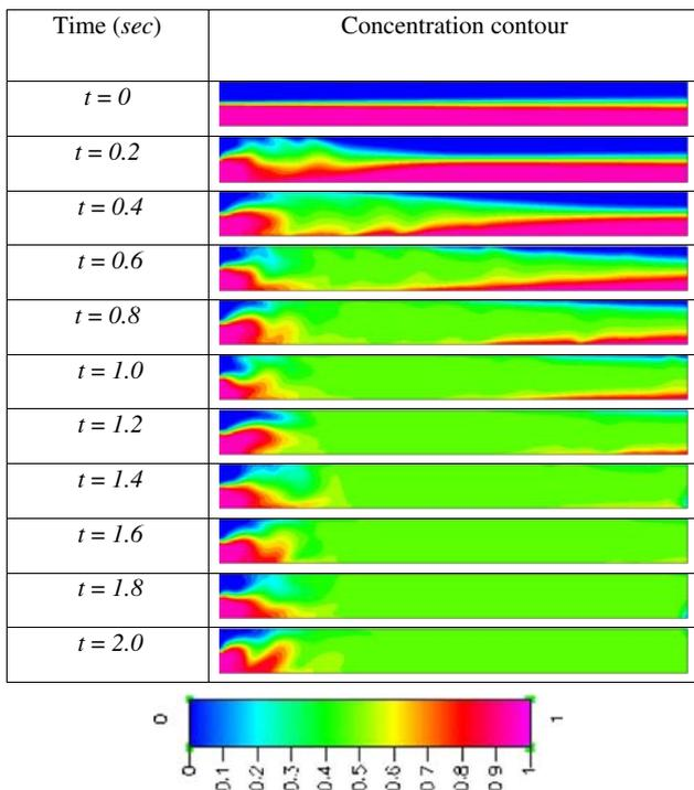
**Fig. 12** Concentration contours at different times in the central plane ( $z = 0$ ) of the mixing channel.  $W = 100 \mu\text{m}$ ,  $f = 25 \text{ Hz}$ . Initially two fluids are mixed by the diffusion only without agitation by particles
