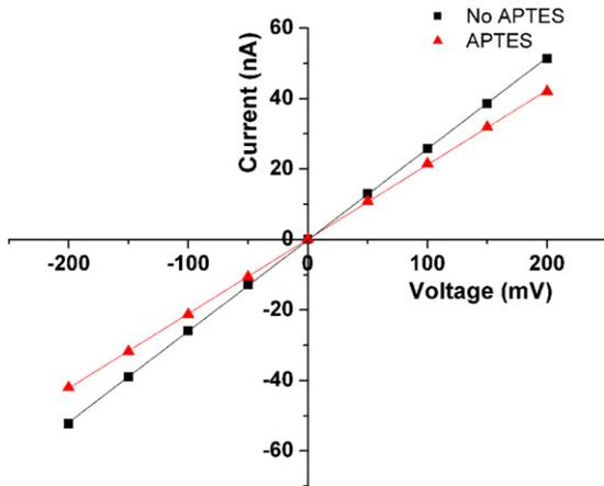
**Figure 5.** *IV* curves were plotted for the nanopore before and after chemical modification by recording the average current at regular voltage steps for a 10 s period. While the *IV* relation remains linear in the tested voltage range, the conductance of the pore was found to decrease from 0.256 to 0.211  $\mu\text{S}$  post-chemical modification.
