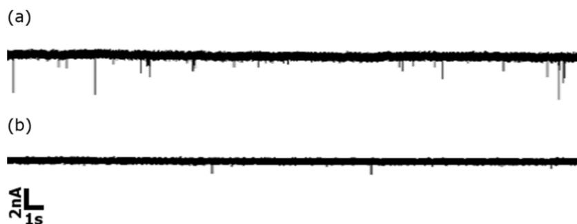
**Figure 6.** (a) Drops in the current across the chemically modified nanopore were observed when the nanoparticle mixture was introduced into the anodic half-cell. The frequency of these events is much higher than that observed with an unmodified pore shown in (b).
