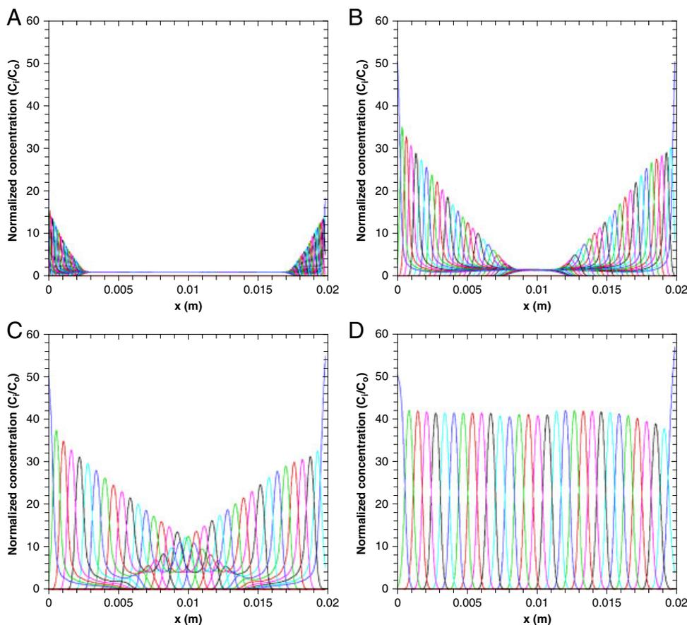
**Figure 4.** Normalized concentration behavior of ampholytes during the IEF process: (A) 50 s, (B) 200 s, (C) 400 s and (D) 1000 s.
