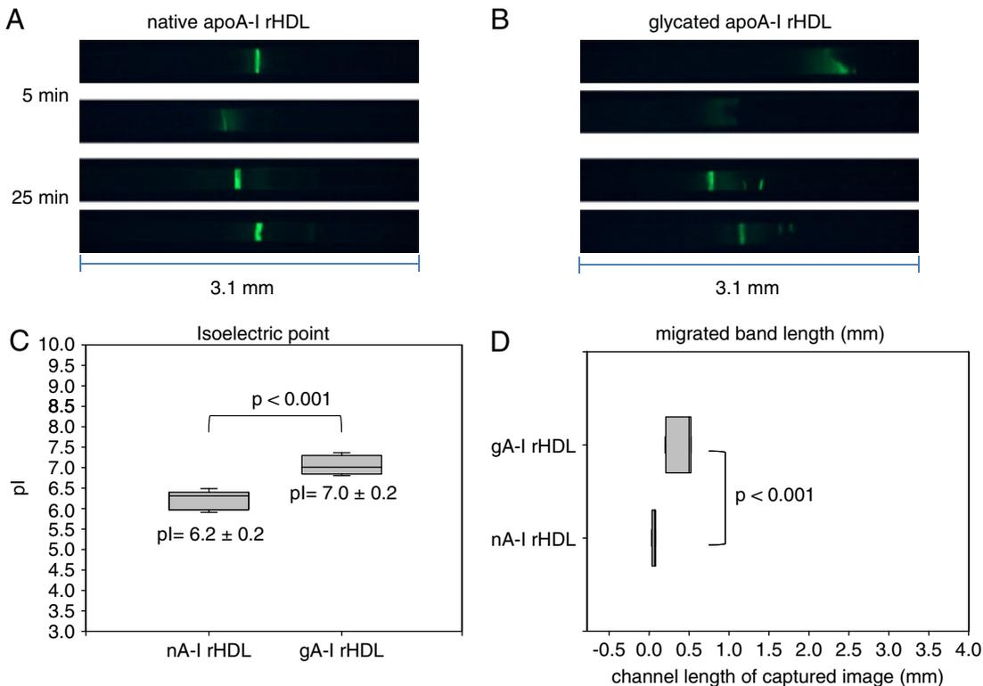
**Figure 6.** Representative image of apoA-I-rHDL migration in microfluidic channel, in the presence of ampholyte (pH 3–10). Fluorescence image of the migration pattern at 5 min (A) and 25 min (B). The distance of migration (C) and  $pI$  range (D) determined from the computational simulation model.
