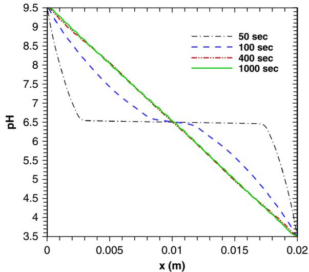
**Figure 5.** Changes in the pH distribution during the ampholytes-based IEF process under the electric potential of 50 V, with 31 ampholytes
