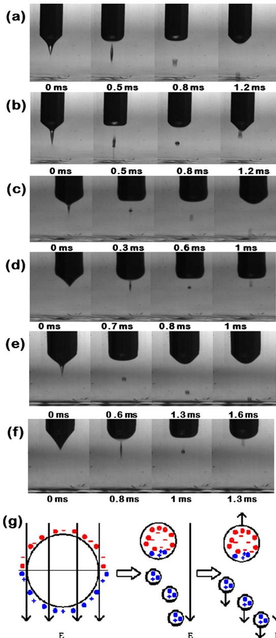
FIG. 2. (Color online) Droplet flight behavior for conductive substrate at different times after forming a droplet. (a) straight flight to the substrate with dc voltage, (b) retreat to the nozzle with dc voltage, (c) straight flight to the substrate with ac voltage, (d) retreat to the nozzle with ac voltage, (e) straight flight to the substrate with SP-ac, and (f) retreat to the meniscus with SP-ac. (g) Mechanism of charge redistribution and breaking of a droplet under a strong electric field.
