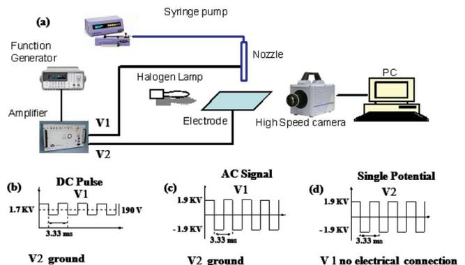
FIG. 1. (Color online) (a) Experiment set up used for EHD printing. External potentials for (b) dc case, (c) ac case, and (d) single potential ac (SP-ac) case.
