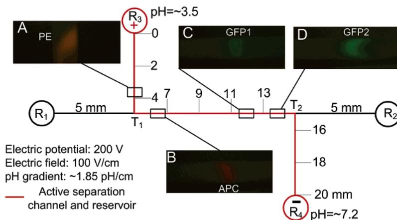
**Figure 5.** Final positions of refocused proteins at the end of second-stage IEF. Experimental conditions were shown in Figure 4. Photos A–D were taken at 780, 840, 850, and 870 s, respectively, after the initiation of the second-stage IEF. Resolution of GFP1 and GFP2 is 4.68, which is 2-fold greater than that at the end of the first stage.
