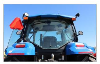
Any time you operate a tractor on a public road, you must ensure the tractor is properly equipped with a slow-moving vehicle emblem and the required lights and reflectors, depending on the time of day and visibility conditions.
