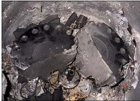
*An unbalanced load and metal fatigue caused this rotor to split in the middle while spinning at 55,000 rpm.*
