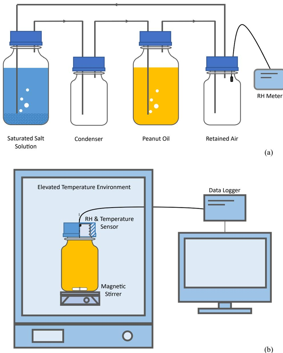
**Fig. 2.** Experimental apparatus for a) rapid water activity conditioning of a large quantity of oil; and b) water activity measurement of oil by analyzing its headspace air with an electrical capacitive sensor.
