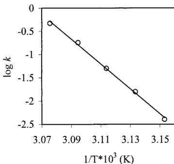
Fig. 3. Arrhenius plot for temperature effects on thermal death rates of fifth-instar Indianmeal moth. Line represents linear regression equation  $\log k = 82.22 - 26.83 \cdot 1000/T$  ( $r^2 = 0.99$ ) where  $t =$  time and  $T =$  temperature.
