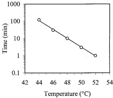
Fig. 2. TDT curve for fifth-instar Indianmeal moth ( $N = 600$ ) at a heating rate of  $18^{\circ}\text{C}/\text{min}$ . Line represents linear regression equation  $\log t = 13.39 - 0.26 T$  ( $r^2 = 0.99$ ) where  $t =$  time and  $T =$  temperature.
