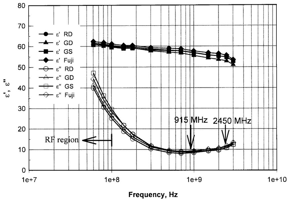
Figure 2—Plot of mean dielectric constant ( $\epsilon'$ ) and dielectric loss factor ( $\epsilon''$ ) for four apple cultivars at 23°C. Data plotted are the mean of surface and core sections of new apples.
