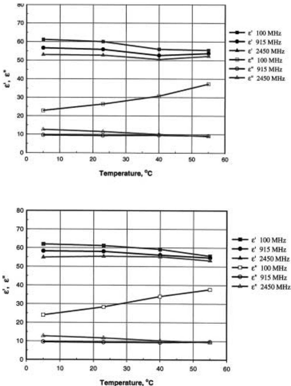
Figure 3—Effect of temperature at given frequencies on the dielectric properties of new (a) GD and (b) ‘Fuji’ apple pulp. Data plotted are the mean of surface and core sections.
